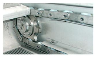
Cog wheel and chain are made of hardened, wear resistant steel that is zinc -galvanized and chromated for long-term corrosion protection; alternatively, wheels and chains can be made of stainless steel
