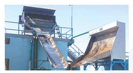
The screen is the only rotary screen available with an automatic doctor blade cleaner assembly that wipes away solids, particularly sticky materials that build up on the primary doctor blade.
